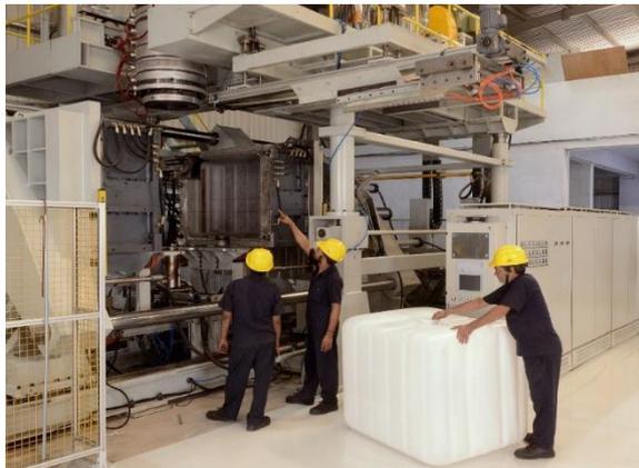
*Manufacturing of rigid Intermediate Bulk Containers*
