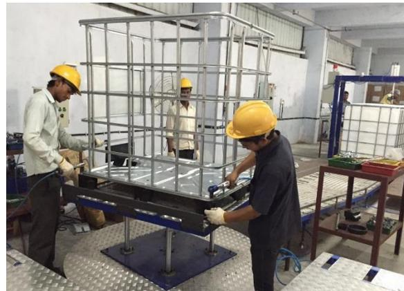
*Manufacturing of cage for rigid Intermediate Bulk Containers*
